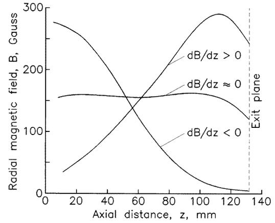
**Figure 7.** Different axial variations in magnetic field strength. (After [37], with permission.)
