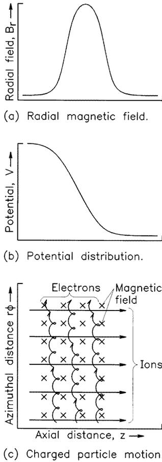
**Figure 4.** Potential distribution and charged particle motion for a given distribution of radial magnetic field.
