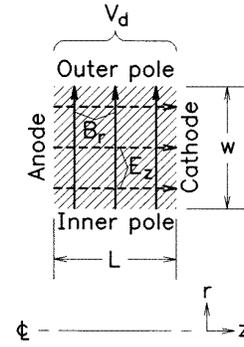
**Figure 5.** Simplified closed drift region (shown crosshatched).
