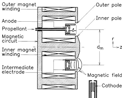
Figure 3. Closed drift thruster of the two stage, anode layer type.
