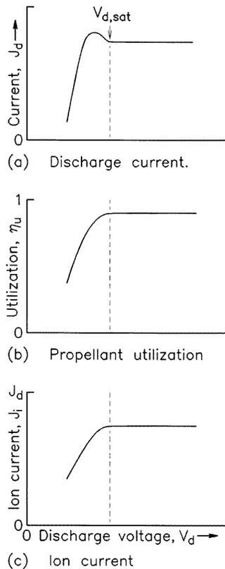
**Figure 13.** Discharge characteristics of a typical magnetic layer thruster at constant propellant flow.
