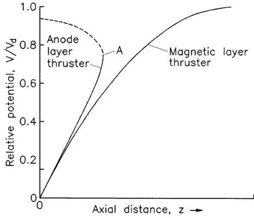
**Figure 11.** Comparison of the potential variations for the discharge channels of anode layer and magnetic layer thrusters. The axial distance shown is measured *upstream* from the exit plane. (After [42], with permission.)
