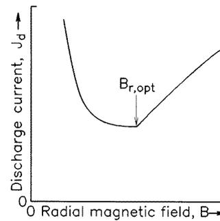
**Figure 12.** Discharge current as a function of magnetic field for a typical magnetic layer thruster at constant discharge voltage and propellant flow.
