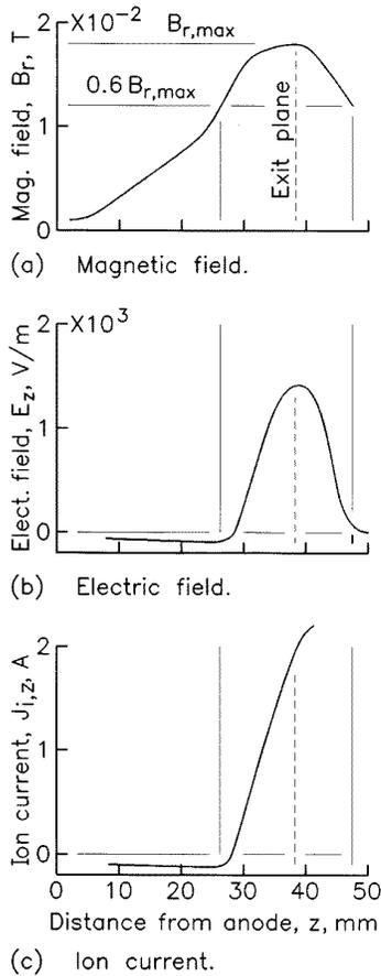
**Figure 10.** Axial distribution of discharge parameters. (After [35], with permission.)
