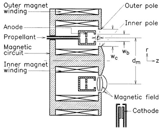
Figure 2. Closed drift thruster of the one stage, anode layer type.
