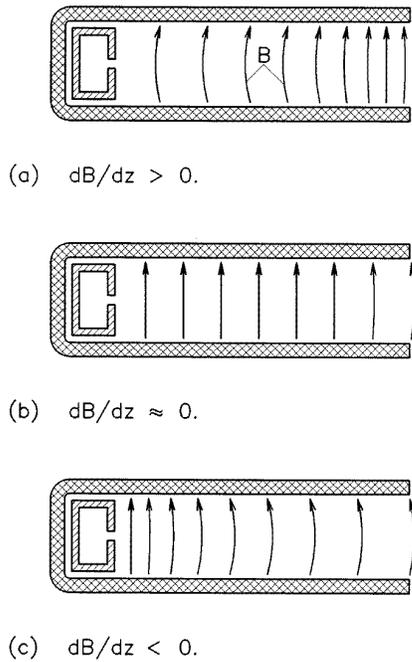
**Figure 8.** Magnetic field shapes for different axial variations of field strength.
