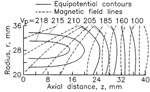
**Figure 6.** Comparison of equipotential contours of plasma potential with the shape of magnetic field lines for a magnetic layer thruster. Xenon flow,  $2 \text{ mg s}^{-1}$ ; discharge voltage, 220 V, magnetic field strength, 150 Gauss. (After [33], with permission.)
