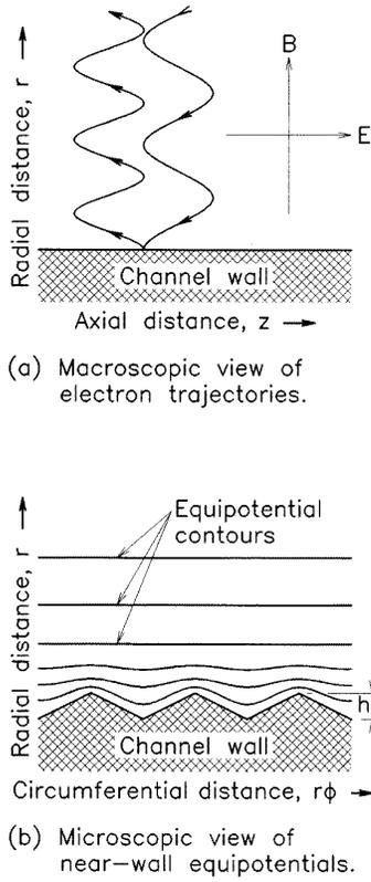
**Figure 9.** Near wall conductivity. (After [39] and [40], with permission.)
